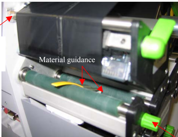
Fig. 2 Print mechanics - upper print unit
